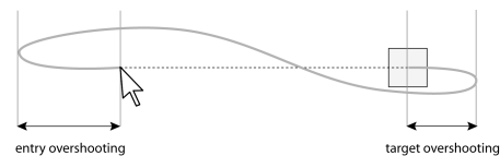
Figure 1. Task axis connecting pointer outcome position and target position on the target display with entry and target overshooting.
